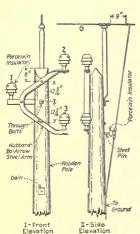
Fig. 150.—Ground wire over a three-phase transmission circuit. (The line wires take the positions 1, 2 and 3.)
